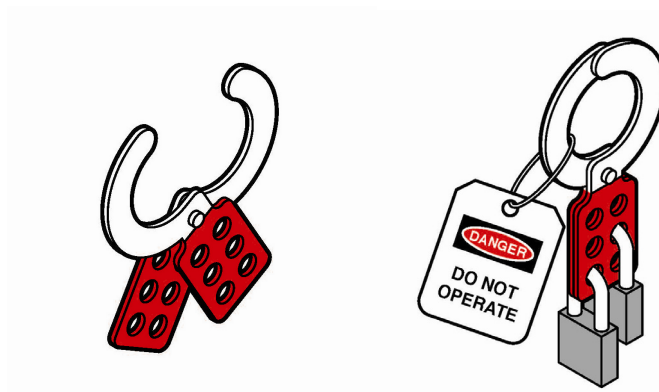
Figure 3: Example of tag and lockout with the padlocks of two workers.
