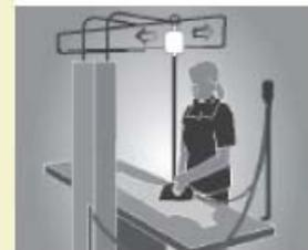
An overhead suspension system reduces the forces required to use the iron.
