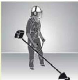
The heaviest part of this brush cutter is located behind the wrists and the weight is supported by a harness.
