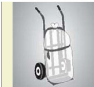
A trolley can eliminate many of the risks involved in manual handling, however, the load will still need to be manoeuvred onto the trolley and through the workplace.
